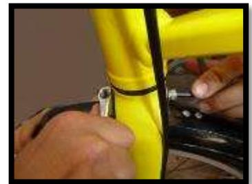
10. Place the saddle and adjust the correct saddle height. Clamp the saddle post.
